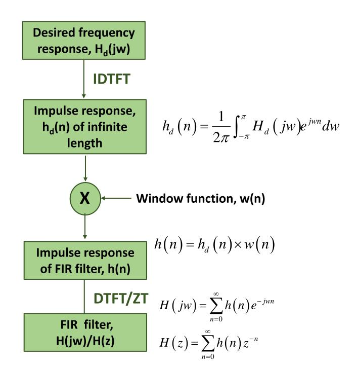
Let  $H_d(e^{jw})$  be the desired response (Typically ideal response). Taking IDTFT on both sides, we get IDTFT $[H_d(e^{jw})] = h_d(n) = \frac{1}{2\pi} \int_{2\pi} H_d(e^{jw}) e^{jwn} dw$ , which gives the impulse response of an IIR filter
