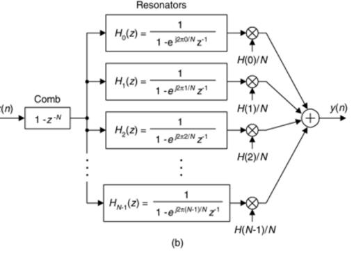
Using Conjugate symmetric property of DFT, we have  $H(N-K) = H^*(k)$ , for k = 0, 1, 2,.....(N-1)/2 when N is odd and  $H(N-K) = H^*(k)$ , for k = 0, 1, 2,.....(N/2)-1 & H(N/2) = 0 when N is even
